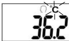
Step 5: No operation in 60 seconds, the device will record the last measuring data and shut down automatically.
