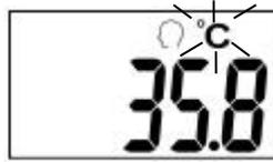
Step 3: Direct the probe to measuring area (Shown in Figure 3.1.1 and 3.1.2), press the “measuring” button till a “Beep” sound from the buzzer. Measuring program starts. Keeping device in position for one second after two “Beep” sounds, the temperature value will show on screen along with the model symbol.
